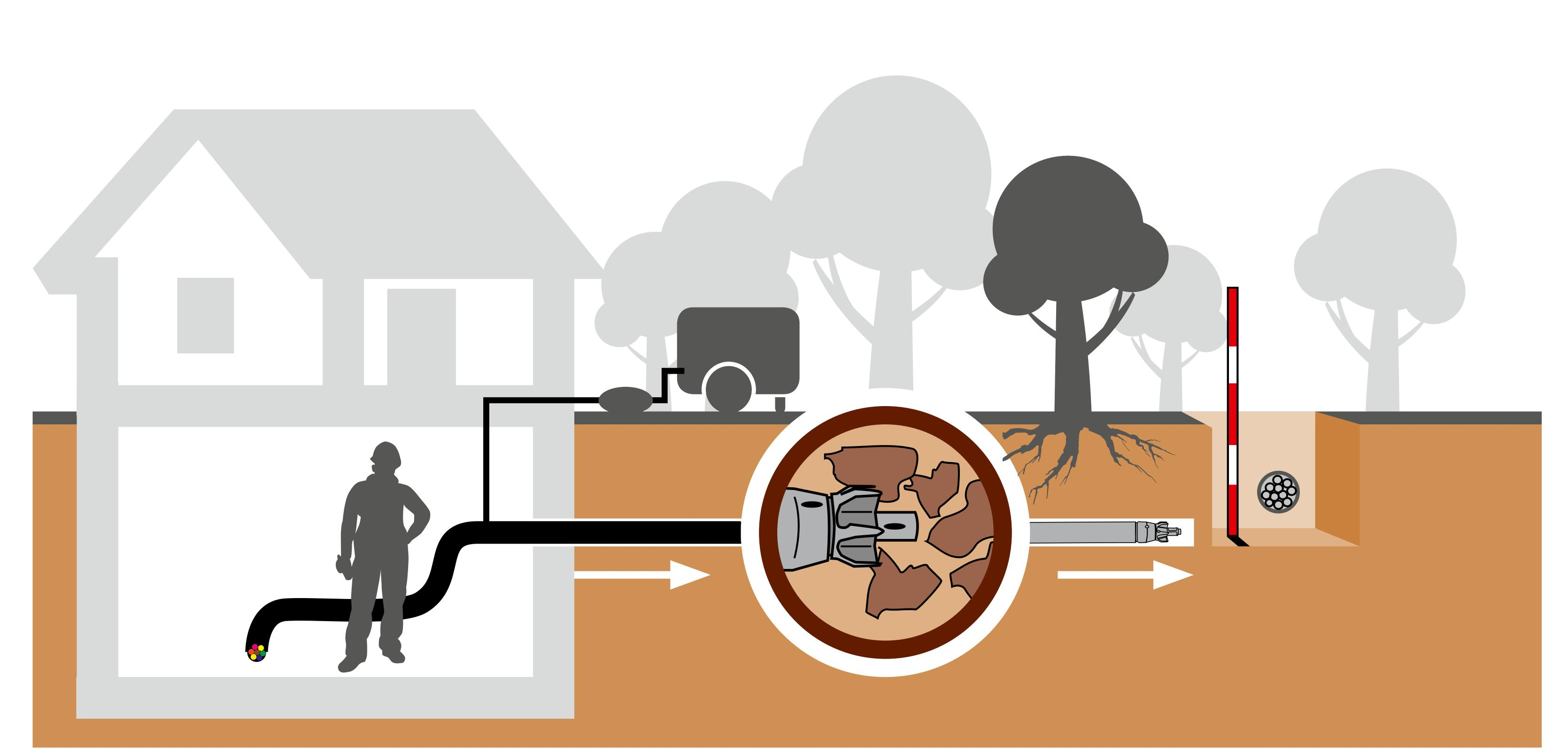
Environmentally friendly installation of FTTH, gas or water service connections without destruction of valuable surfaces
