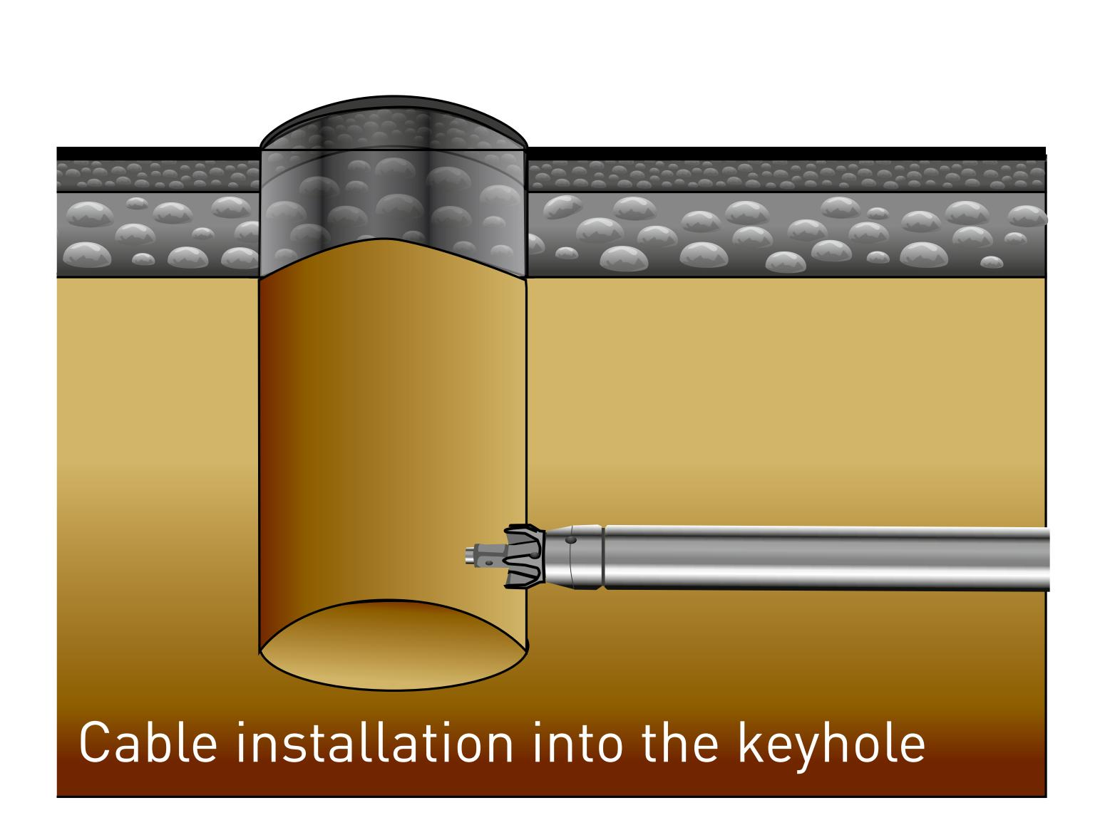
Fast and safe connection to the power grid using the keyhole technology
