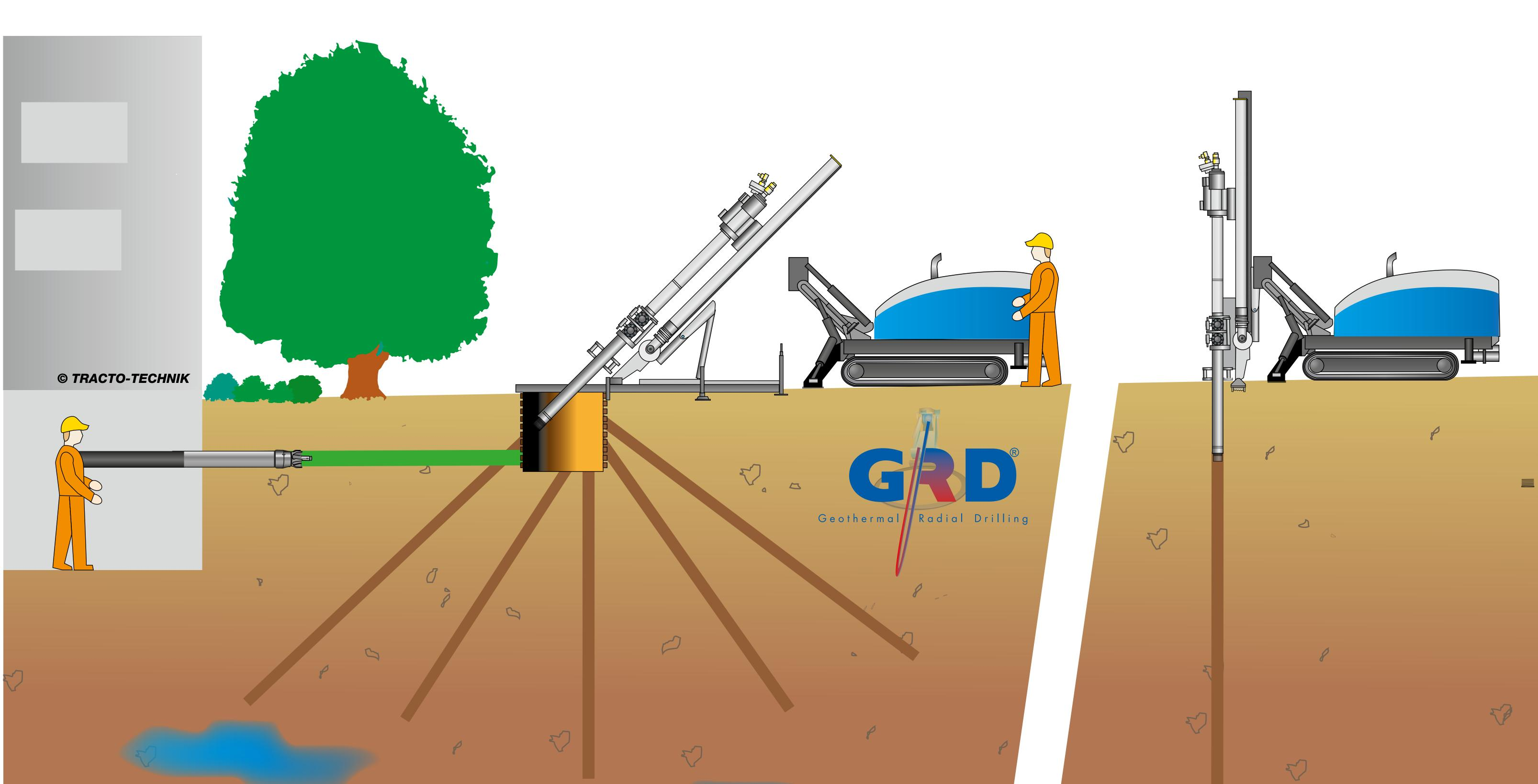
Horizontal and vertical heat exchangers installed in the most confined innercity spaces
